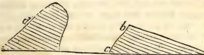
The nature of the rock, and the thickness and direction of the strata, prove that they are the same formation, and that the intervening mass has been removed by some local causes. When strata terminate abruptly, they are said to end in an *escarpment*, as at *b c*. When rocks present nearly perpendicular faces, they are said to form *mural* or wall-like precipices.
